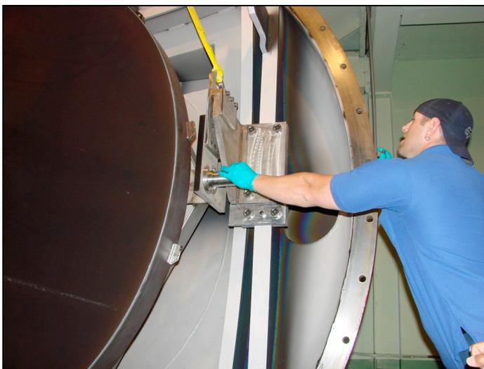
**Load the optic into the tank**
