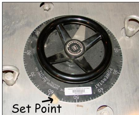
As with the previous power-stat, ramp up slowly from zero to the set point. Hold there till the amperage meter starts to spike then back off enough to keep the meter around the set point amperage.
