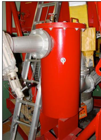
Climb the ladder enough to remove the cover from the trap and fill the center hole of the trap with the dry ice. Use the stick that is located by the trap to tamp the ice periodically to keep the ice in good contact with the sides of the trap.
