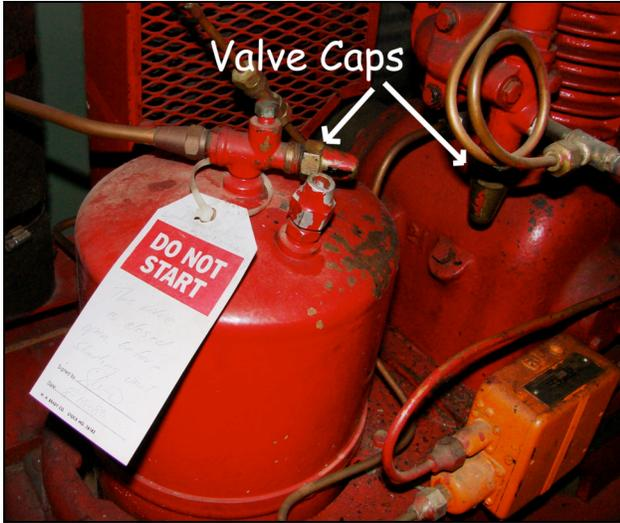
Remove the valve caps and using a refrigeration wrench open the valves.
