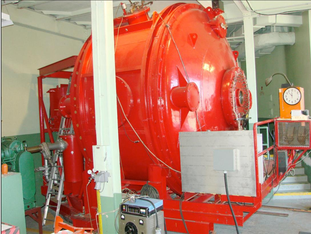
**Introduction:** This chamber is used for coating our Mountain optics. Our plans are to send most optics 40" and smaller to the coating chamber in Santa Cruz where they can do special coatings. We only coat with aluminum here and we no longer use SiO overcoating because of the light loss from this coating.
