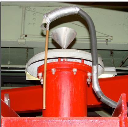
When the DP's are opened its time to fill the tank cold trap with liquid nitrogen. This trap is located on top of the DP valve chamber.
