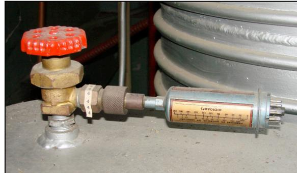
The readout for the thermocouple gauges is in the rack at the operator platform. Turn on the toggle switch and set the rotary knob to the TC you want to read out. The gauge reads out in microns.
